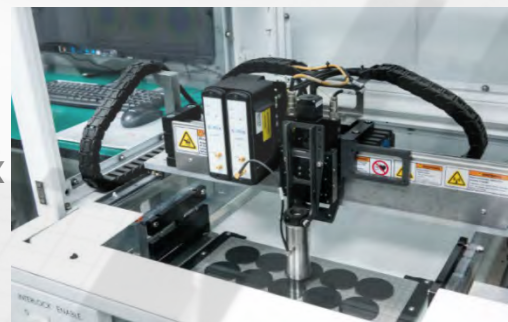
Step 7: Ultrasonic scanning inspection
