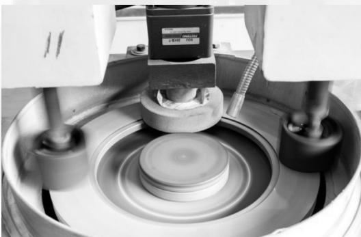
Substrate face polishing and growth face lapping
